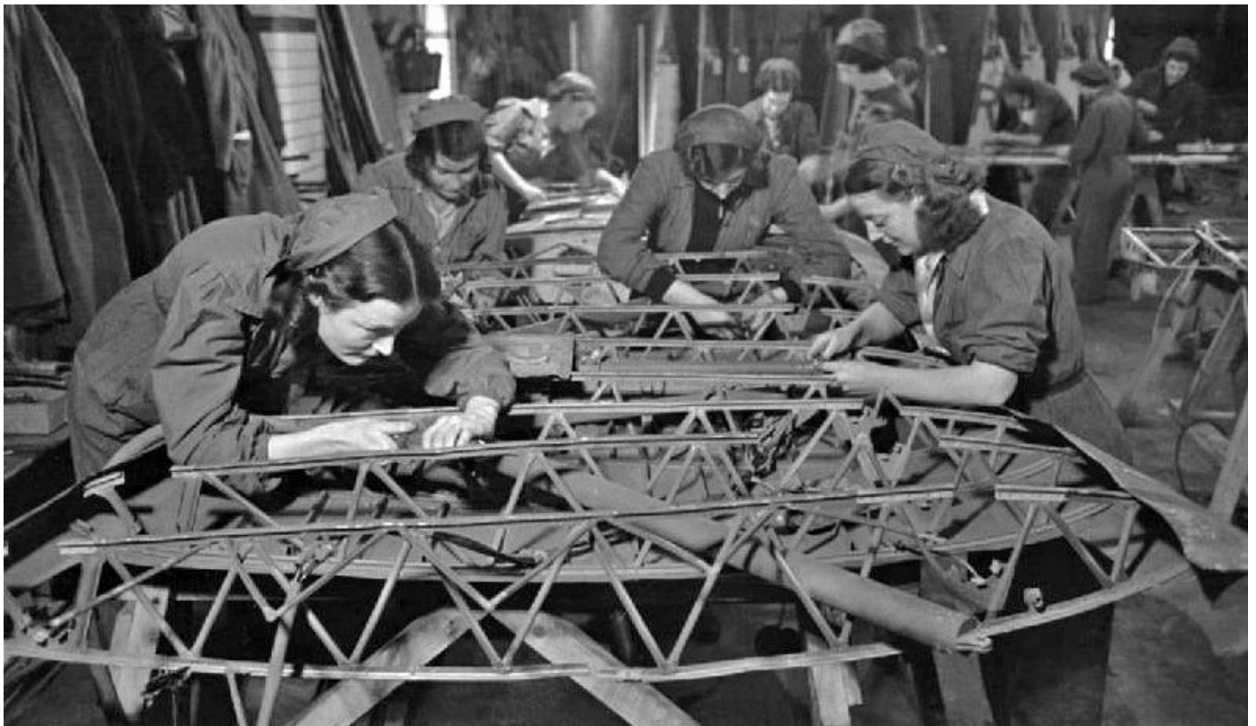
Women repairing a wing of a Fairey Swordfish aircraft – Author, United Kingdom, Imperial War Museum, Public domain, Wikimedia
