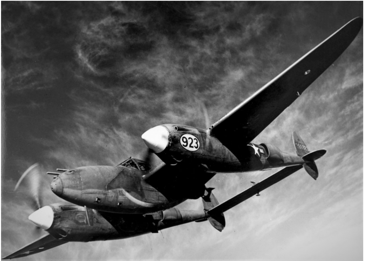
Lockheed P-38 Lightning fighter-bomber capable of carrying 2,000 pound bomb pay loads – Author, U.S. Air Force, Public domain, Wikimedia
