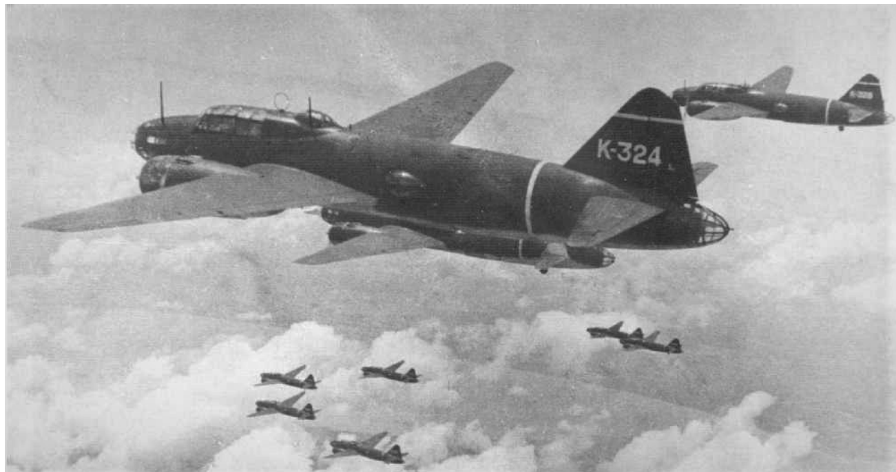
Mitsubishi Betty G4M1 bombers – Unknown author, Public domain, Wikimedia. Designed for high speed and long range, to reduce weight and increase range, the Mitsubishi chief designer Kiro Honjo did not use self-sealing fuel tanks and armor plating to protect the crew, leaving the craft vulnerable to cannon fire of the P-38s during 'Operation Vengeance.'
